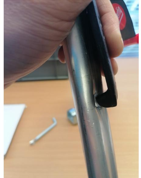
1. Loosen the clamp using a flat screwdriver to remove the 'key' supplied. (keep this key as it can be used from this point on to remove/attach the blade) Then slide the loose clamp back up the handle.
